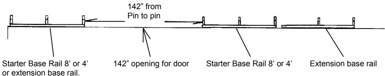
Anchor base rails with 1/2" x 7" concrete wedge anchors in all anchor holes. See your building instruction manual for details.
