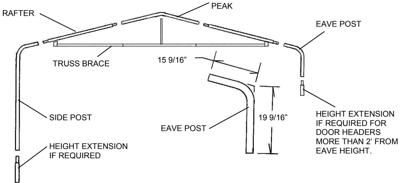
**STEP 7: INSTALLING THE TWO SPECIAL ROOF/WALL FRAME SECTIONS IN SIDE DOOR BAYS.**
